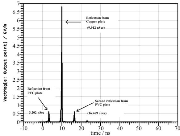
Fig. 2. Reflections from copper and PVC plates
