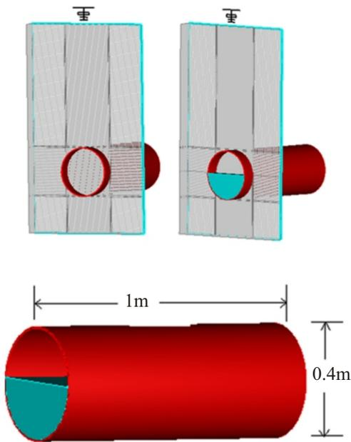
Fig. 5. Simulation setup of second case
